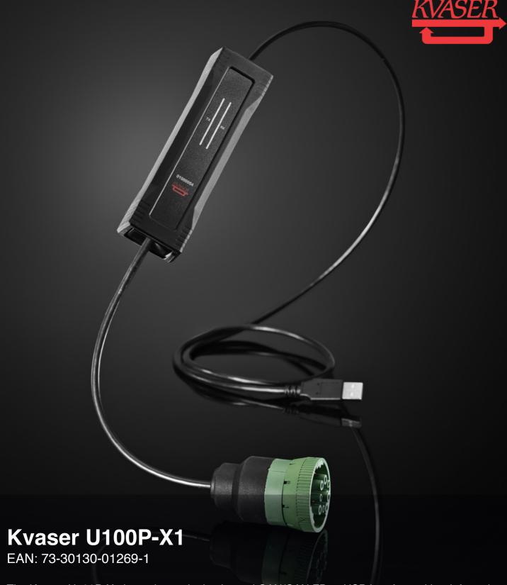
The Kvaser U100P-X1 is a robust, single-channel CAN/CAN FD to USB interface with reinforced galvanic isolation (Tested according EN 60335) that squarely addresses the needs of the evolving automotive development market. Fully compatible with J1939, CANopen, NMEA 2000® and DeviceNet, this is the first in a new range of interfaces that is also suited to rugged applications in marine, industrial, heavy duty vehicle and heavy industries.
