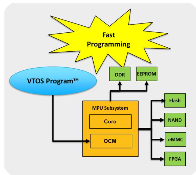
VTOS Program is a bare-metal application that requires no other software, operating system, or boot loader – making VTOS Program an excellent solution for new boards with no software, or boards that will not boot.
